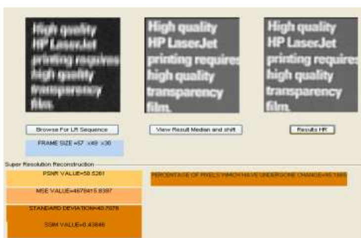
Fig.9. GUI wit HR result and different calculated image quality parameter for Printer text test vector
