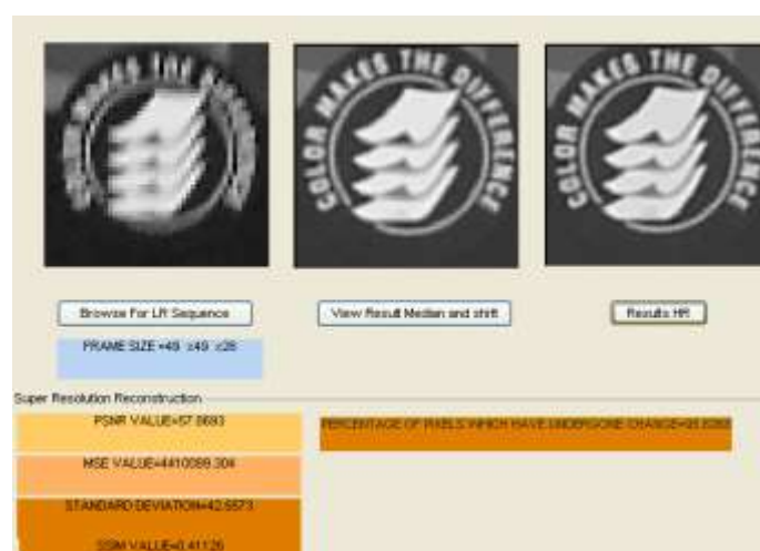
Fig.10. GUI wit HR result and different calculated image quality parameter for disk test vector
